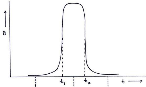
Figure 7.5: Variation of  $B$  at the coil with time
