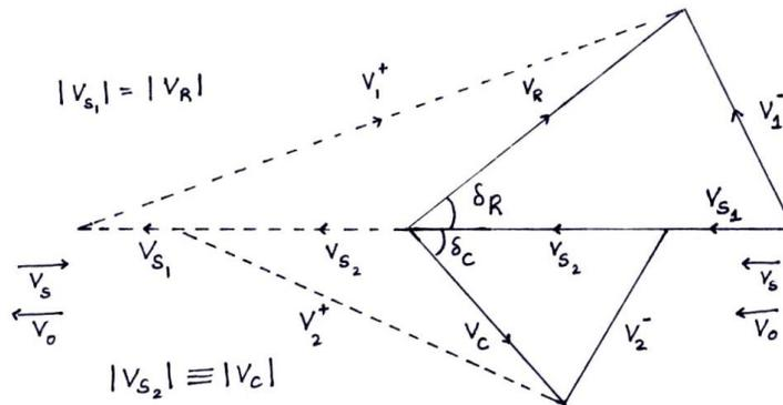
Figure 2.5: You can see that (a)Phase of  $V_R$  (or  $V_C$ ) is same relative to  $V_s$  and  $V_C$  (b)  $\delta_{RC} = \delta_R + \delta_C$
