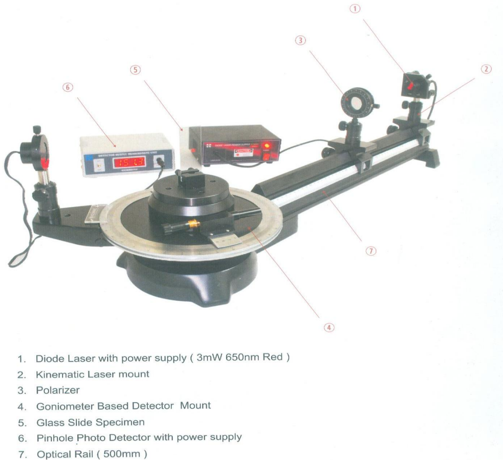
Fig. 4: Experimental setup for Brewster angle measurement.
